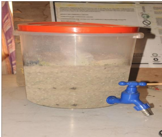
Figure 1: Surface water treatment with sand filter
