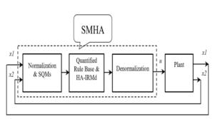
*Figure 1. Diagram of control system using HA [12]*
