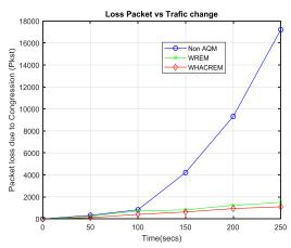
Figure 6. Cumulative packet loss as the source of information increases
