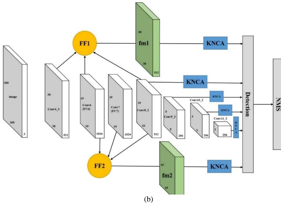
Figure 1. (a) is the SSD framework, (b) is our FFASSD framework.
