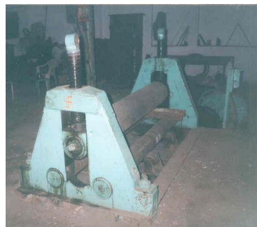
Figure 1: Power operated Sheet Metal bending machine showing roller and adjustable screw arrangement
