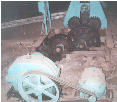
Figure 2: Power operated Sheet Metal bending machine showing gear arrangement with motor
