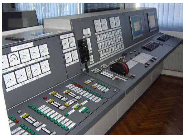
Figure 6. Full mission engine room simulator Kongsberg ERS-L11 MAN B&W-5L90MC-VLCC Version MC90-IV
