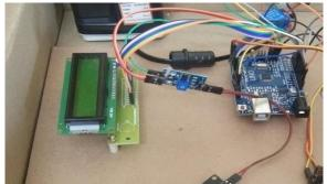
Figure 16 Interfacing of Arduino with LCD
