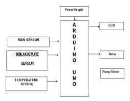
Figure 11. Interfacing of Devices
