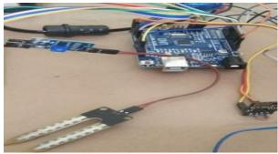
Figure 13 Interfacing of Soil Moisture Sensor
