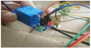
Figure 14 Interfacing of Relay
