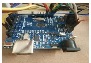
Figure 2. Arduino Uno Board
