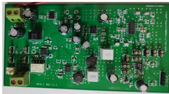
Fig. 11. The fabricated circuit of the proposed capacitive sensor
