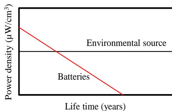
Fig. 1: Continuous power vs. Life for several power sources [9].
