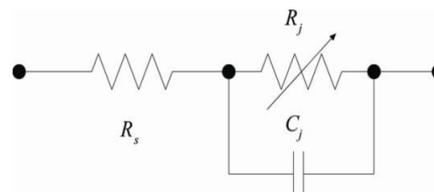
Fig. 3: SPICE model of Schottky Diode [11].
