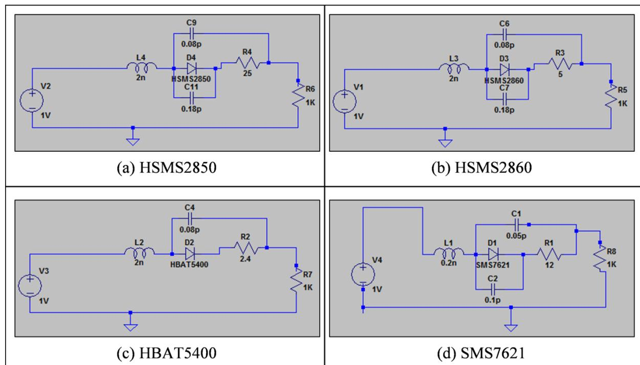
Fig. 4: Models of selected Schottky diode in LTSpiceIV.
