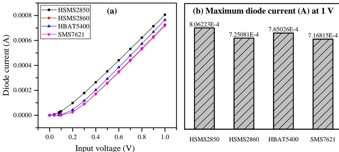
Fig. 6: (a) I-V characteristics of diodes, (b) Maximum diode current at 1 V input voltage.
