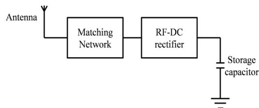
Fig. 2: Block diagram of RF Energy Harvester.
