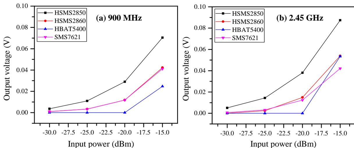
**Fig. 7:** Output voltage characteristics of the selected Schottky diodes at low input power levels - (a) Output voltage of diodes at 900 MHz frequency, (b) Output voltage of diodes at 2.45 GHz frequency.
