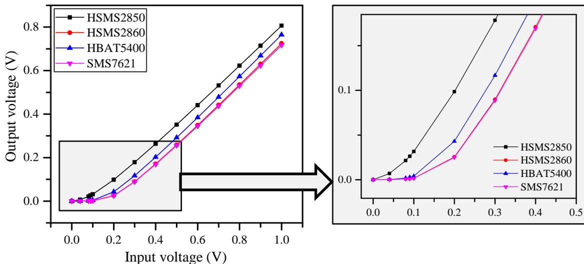
Fig. 5: Comparison of turn-on voltage characteristics for selected Schottky diodes.
