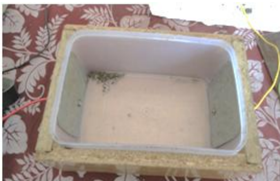
Figure 2: Test box for soil resistivity measurement
