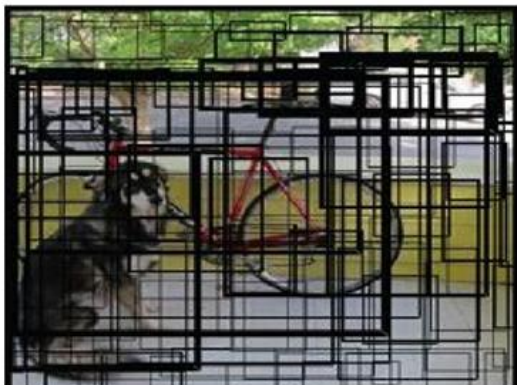
Fig 2.1(b) Calculate bounding boxes and confidence score for each box.
