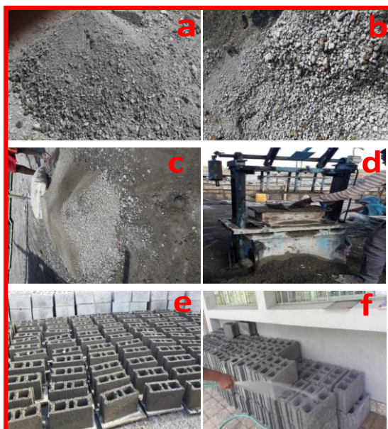
Fig-2 (a) Concrete waste material, (b) Light weight aggregate (c) Dry mixture of CWM and LWA (d) molding of HCBs (e) HCB after casting (f) HCB for Curing.
