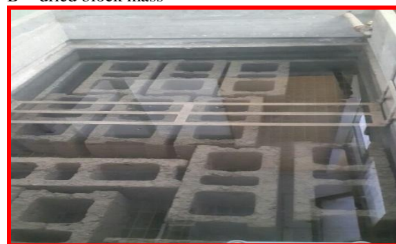
Fig-3 HCB immersed in water for water absorption test.
