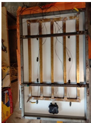
Fig. 1. PV panel Setup with (C-TYPE) cooling
