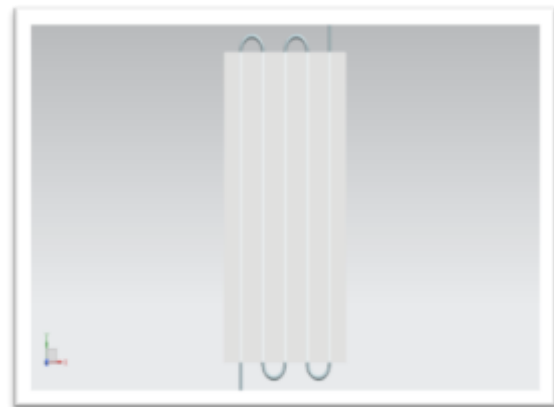
Fig.12.Solar Panel with tubes
