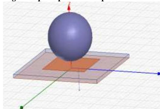
**Fig 15:** Spherical Lens using Square patch
