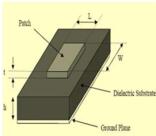
**Fig 1.** General structure of microstrip patch antenna
