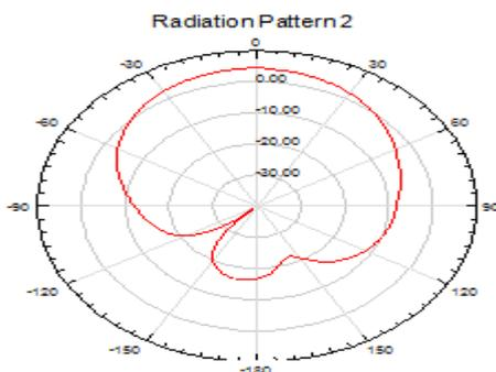
Fig 6. At phi -90 degree Freq – 5.5GHz
