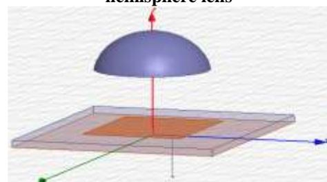
**Fig 2.** Hemisphere lens with Rectangular patch
