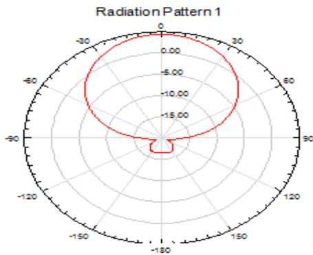
**Fig 10:** At phi -0 degree Freq – 5.5GHz
