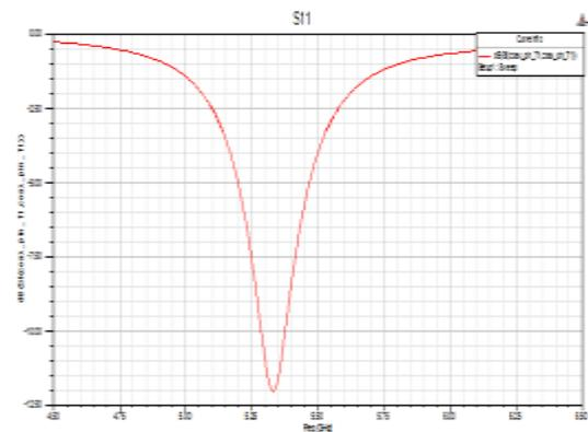
Fig.8 : Simulated Return Loss
