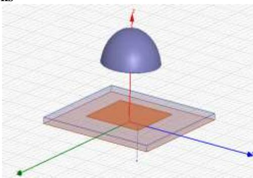
**Figure 12:** Design of Hemispherical lens with square patch
