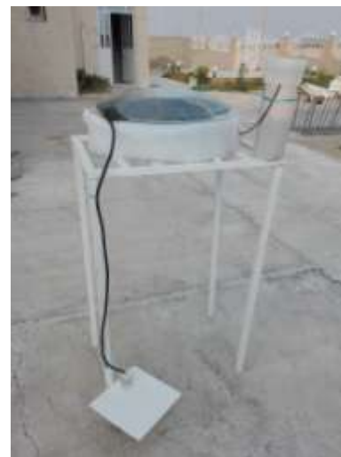
Fig. 2. A photograph of the fabricated hemispherical solar still
