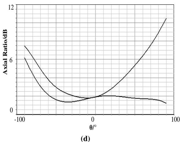
**Figure 8. Simulation results of the 2\*2 pentagon micro-strip antenna array:**
