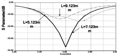
Figure 5. Simulated S parameter for feed points
