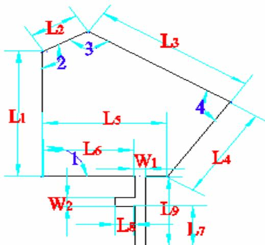
**Figure 2. Side length of the pentagon antenna**
