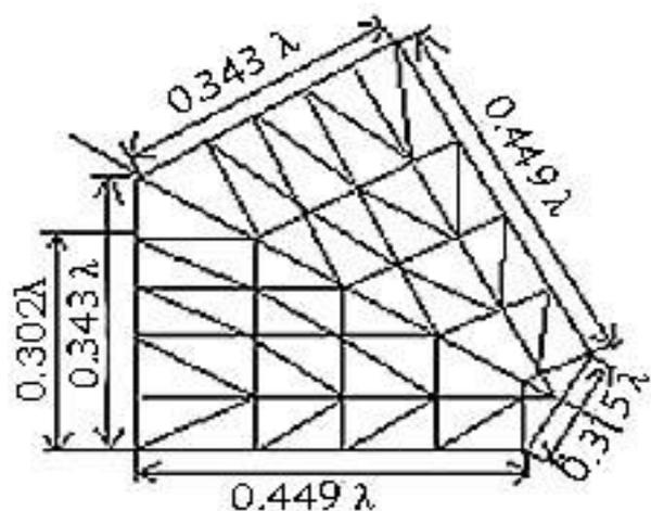
Figure 1. Pentagon Micro-Strip Antenna units Divide
