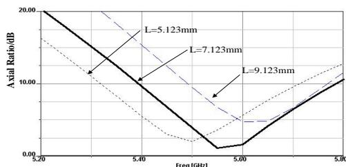
Figure 3. Simulated axial ratio for feed points.
