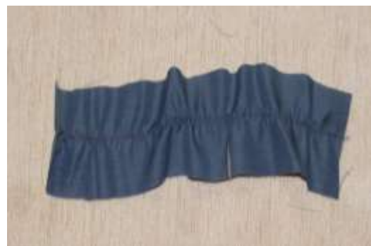
(Fig.No.1- Occurrence of Seam Puckering)
