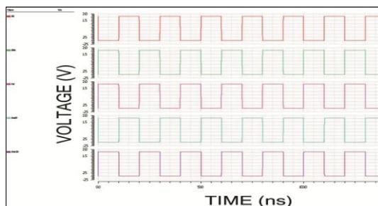
**Figure 5(A):** Transient Response Of 6T SRAM I 45nm
