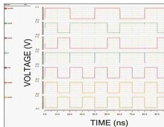
**Figure 7(C):** Transient Response Of 8T SRAM In 90nm
