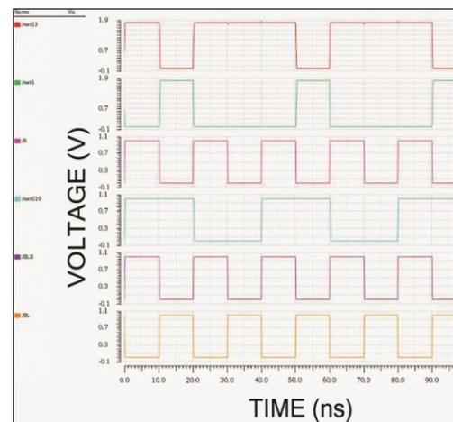
**Figure 7(B):** Transient Response Of 7T SRAM In 90nm
