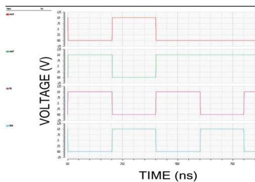
**Figure 6(D):** Transient Response Of 9T SRAM In 65nm
