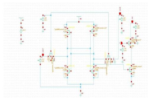
**Figure 3 :** Eight Transistor (8T) SRAM
