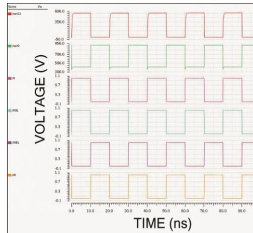
**Figure 7(A):** Transient Response Of 6T SRAM In 90nm
