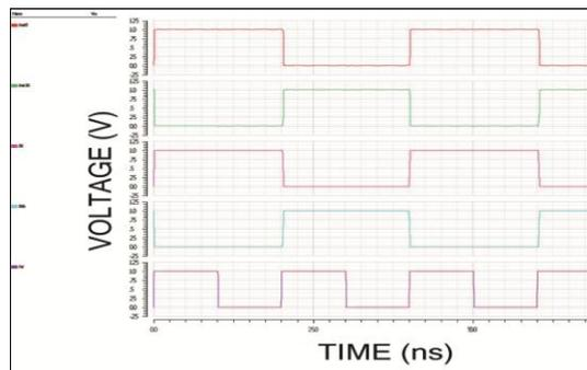
**Figure 6(A):** Transient Response Of 6T SRAM In 65nm
