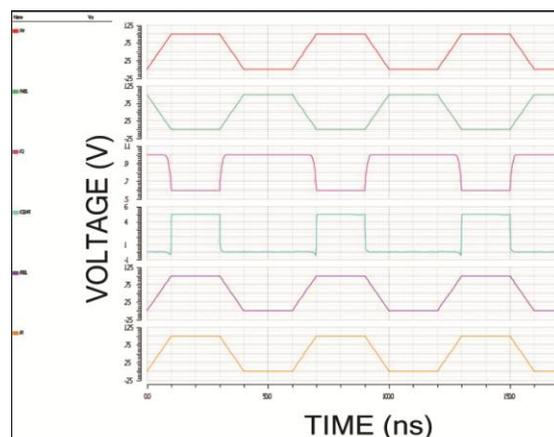
**Figure 5(B):** Transient Response Of 7T SRAM In 45nm
