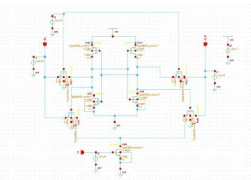
**Figure 4:** Nine Transistor (9T) SRAM
