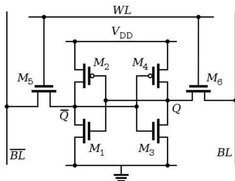
**Figure 1:** Conventional 6T SRAM
