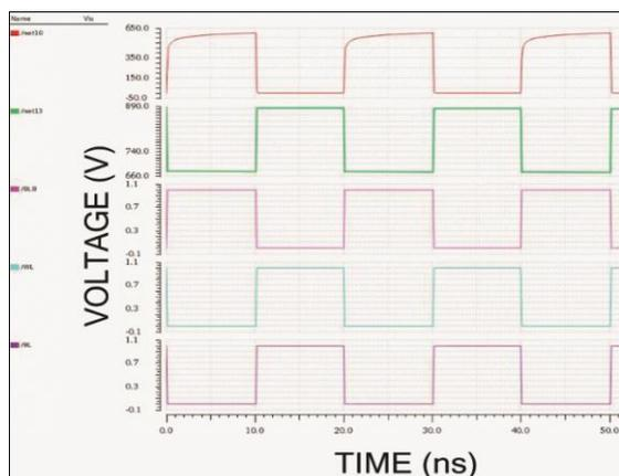
**Figure 7(D):** Transient Response Of 9T SRAM In 90nm
