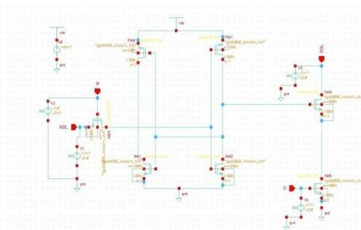
**Figure 2:** Seven Transistor (7T) SRAM
