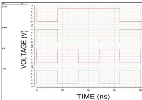
**Figure 6(B):** Transient Response Of 7T SRAM In 65nm
