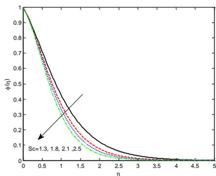
**Fig. 22.** Impact of  $Sc$  on  $\phi(\eta)$
