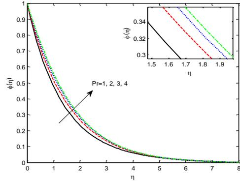
**Fig. 18.** Impact of  $Pr$  on  $\phi(\eta)$
