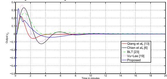
Fig.3.4 Second output response to a unit step in the first input for example 3.2
