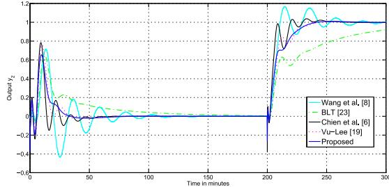
Fig.3.2 Second output response for example 3.1
