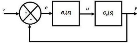
Fig 2.1: Structure of the feed-back control systems
