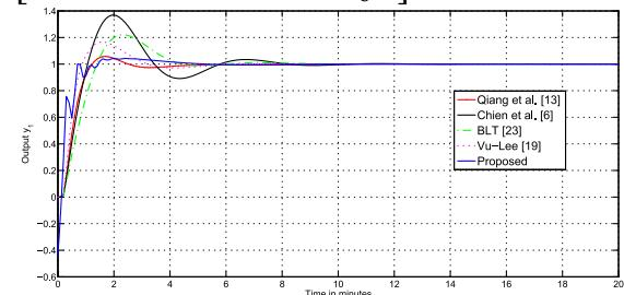
Fig.3.3 First output response to a unit step in the first input for example 3.2
