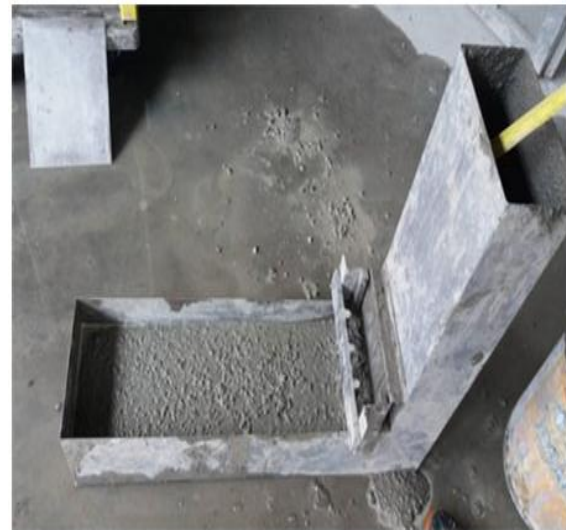
Figure No. 4 – L-Box Test
