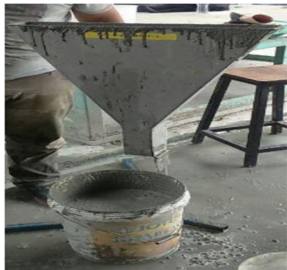
Figure No.2: V-Funnel Test
