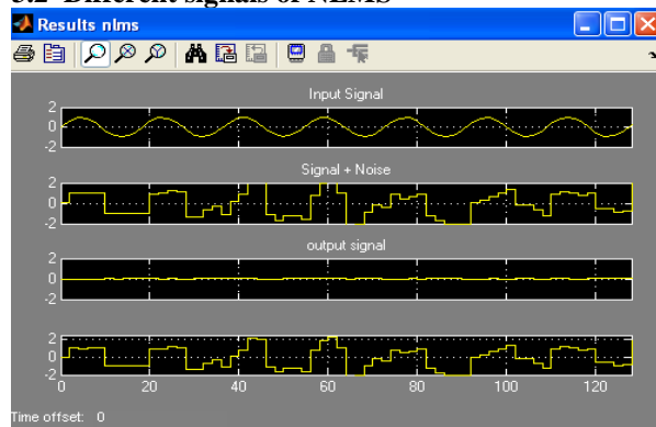
Fig(6): shows input, signal +noise, output & error signal of normalized LMS
