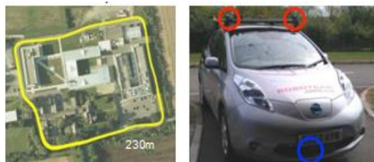
Fig. 3. Experimental test site and platform. The experimental data consists of 24 loops around an urban environment for a total distance of 16km over a period of 24 hours, with images captured at 71 distinct locations along the route. The experimental platform
