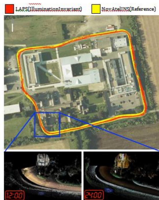
Fig. 6. Metric global localisation results over a 24 hour period using LAPS. Using two Grasshopper2 monocular cameras and two 3D coloured pointcloud scene prior surveys (one
