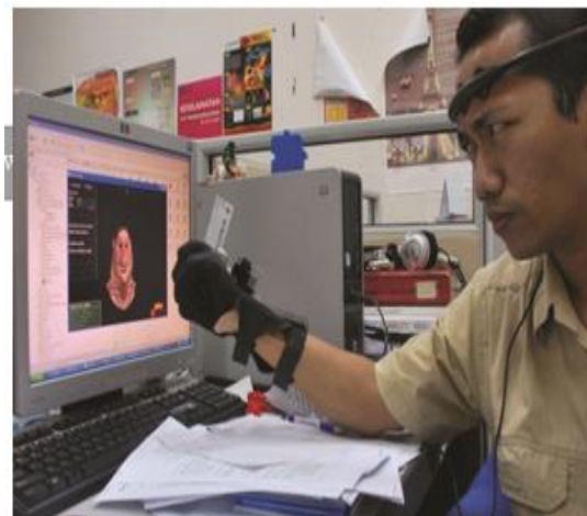
Figure 22. Controlling expression and mode of walking, indicating anger, through mind controller and hand glove
