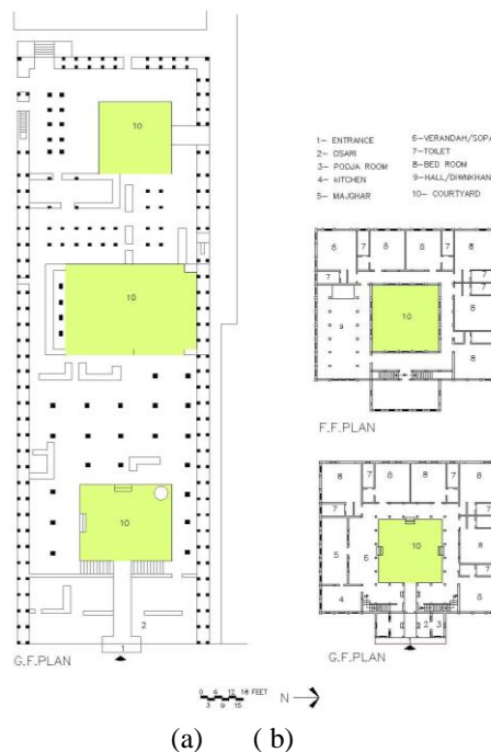
Figure 2 (a) Plan form of Vishrambaug Wada (Traditional Case) (Source: Gupta R.R. 2013,pp.71) (b) Plan form of Dhepe Wada (Contemporary Case)
