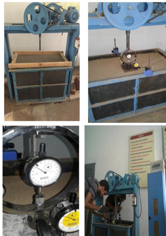
Fig 3.1 Experiment on Square Footings at u/B ratio 0.25 & 0.50
