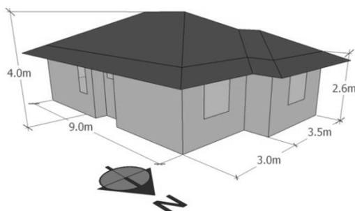
Figure 4 – Isometric view of the baseline model.
