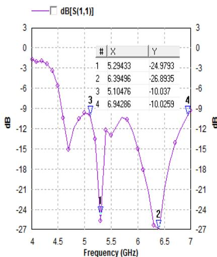
Figure 3: Variation of Reflection Coefficient v/s Resonance Frequencies of SEGCRSMPA with 0.2 mm air gap coupling
