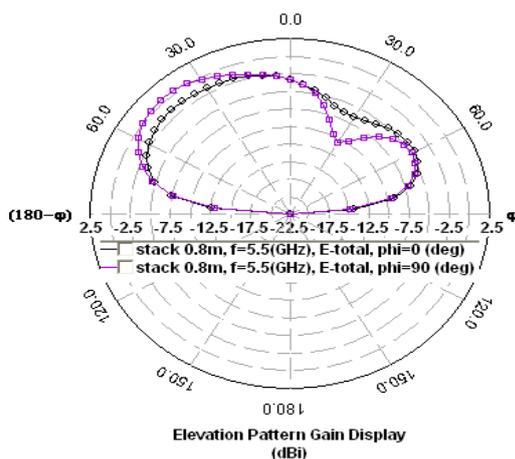
Figure 10: 2D polar Radiation pattern at 5.5 GHz
