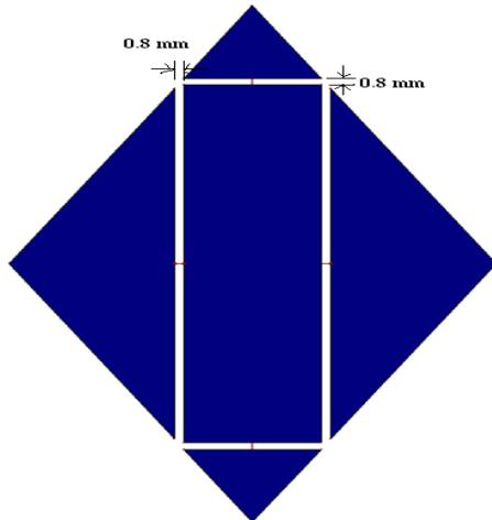
Figure 2: Structure of EGCRSMPA with 0.8mm gap coupling
