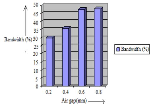
Figure 12: Graph comparing bandwidth of proposed antenna with respect to air gap coupling
