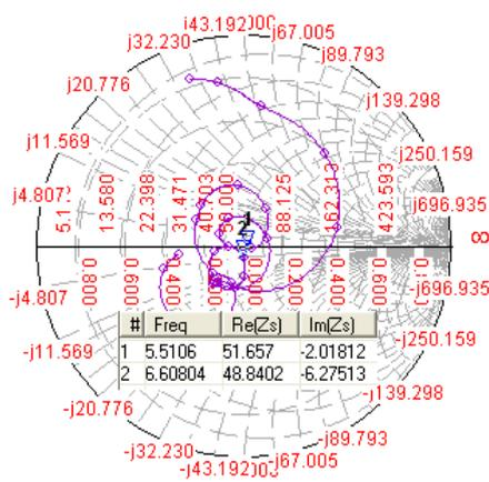
Figure 5: Smith chart for SEGCRSMPA with 0.8mm air gap coupling
