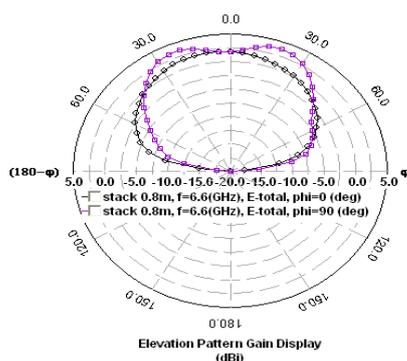
Figure 11: 2D polar Radiation pattern at 6.60 GHz
