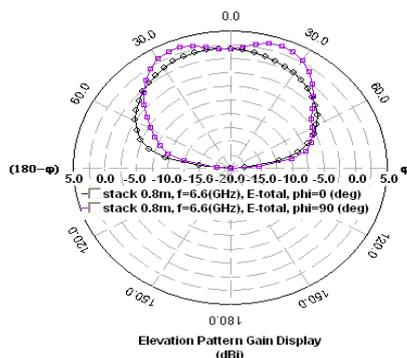
Figure 11: 2D polar Radiation pattern at 6.60 GHz
