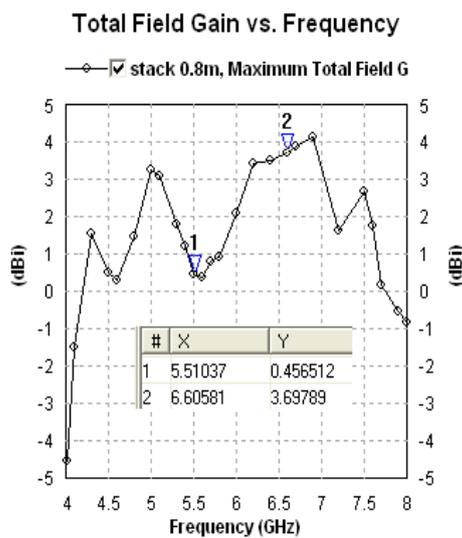
Figure 6: Variation of gain v/s resonance frequencies
