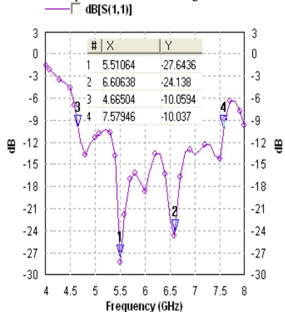
Figure 4: Variation of Reflection Coefficient v/s Resonance Frequencies of SEGCRSMPA with 0.8mm air gap coupling.
