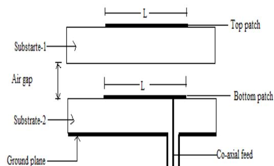
Figure 1: Cross section view of the proposed antenna
