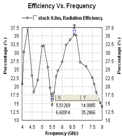
Figure 8: Curve between radiation efficiency and resonant frequencies
