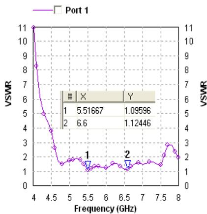
Figure 9: Curve between VSWR and resonant frequencies
