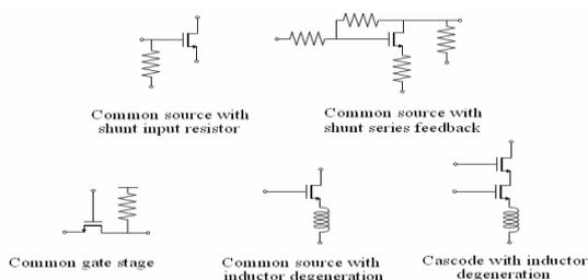
**Fig.1.** Low Noise Amplifier Topologies
