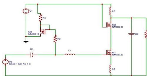
**Fig.2.** Schematic of LNA
