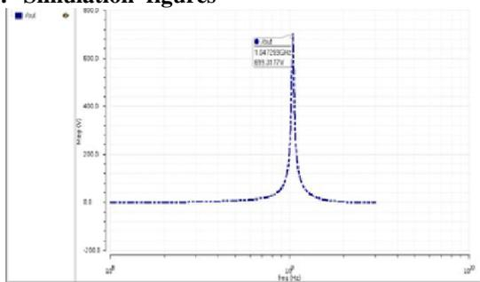
**Fig.4.** Plot for frequency response of LNA at 180nm Technology
