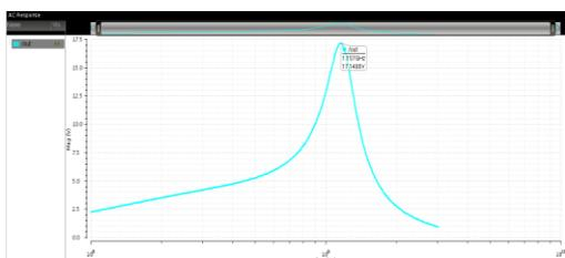
**Fig.5** Plot for frequency response of LNA at 90nm Technology
