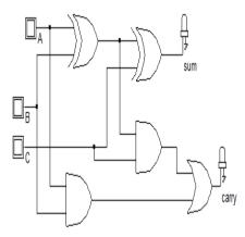
Fig.2Logic diagram of basic full adder
