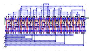
Fig.4.layout design of basic full adder based comparator
