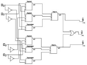
Fig.3.Logic diagram of basic full adder comparator
