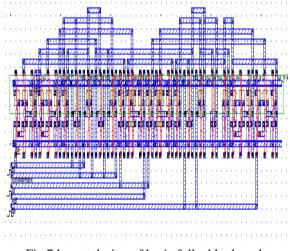
Fig.7.layout design of basic full adder based comparator
