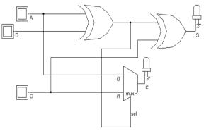
Fig.5.logic diagram of hybrid FULL ADDER
