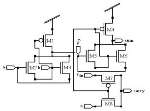
Fig.9.Logic diagram of 8transistor full adder
