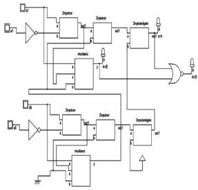
Fig.6.Logic diagram of basic full adder comparator
