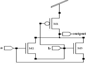
**3T X-NOR GATE** Fig.8.Logic diagram of 3t x-nor gate
