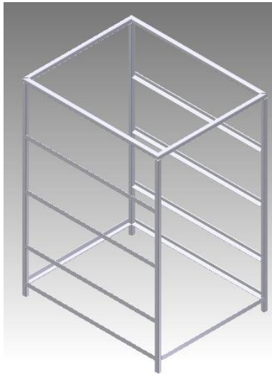
Fig. 2: Cabinet frame work
