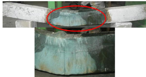
Figure 9b: Flexural Failure and Debonding of Fabric of Beam C2Y
