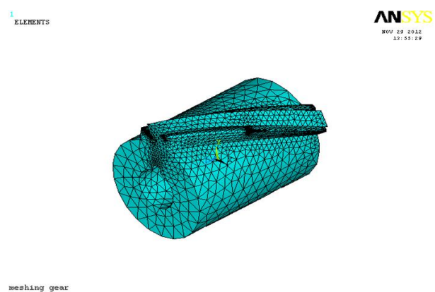
Fig 3 Meshing of Contact gear model
