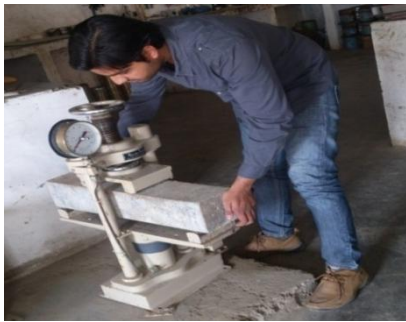
Figure-5: Beam Specimen Third point loading arrangement. (Flexural strength test).
