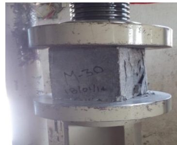
Figure-6: Cube Specimen compressive strength test.
