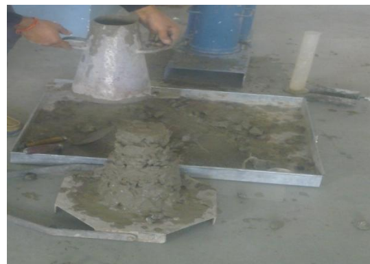
Figure-2: Slump cone test (workability)
