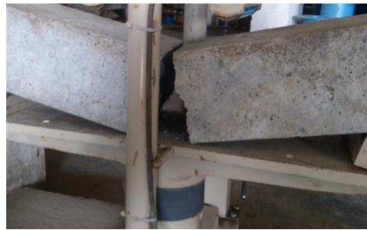
Figure-5: Beam Specimen Third point loading arrangement. (Flexural strength test).
