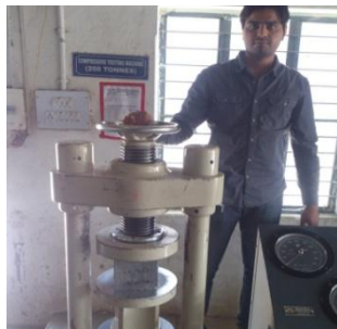
Figure-6: Cube Specimen compressive strength test.
