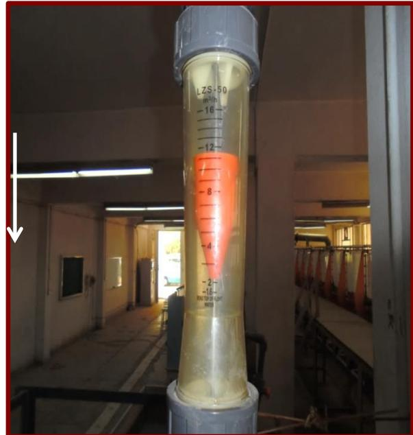
Fig. (4) Ground flow meter and intake flow meter for measuring the intake discharge.
