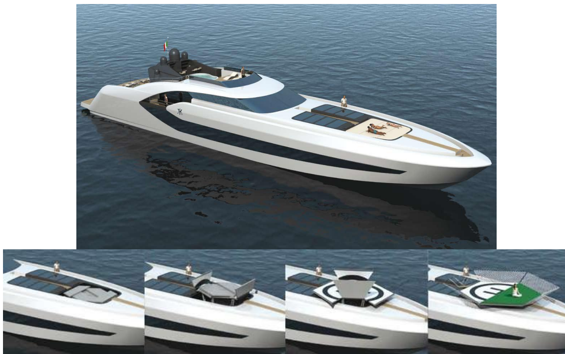
Figure 2. Platform installation example, showing the lifting and opening sequence.
