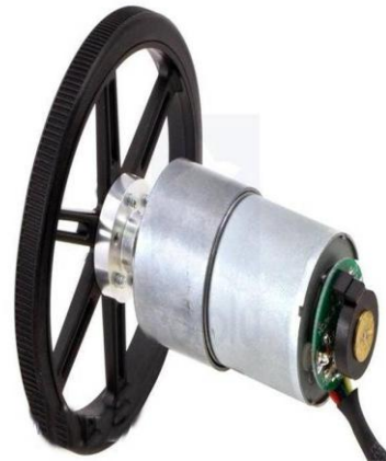
Figure 4: Geared DC Generator
