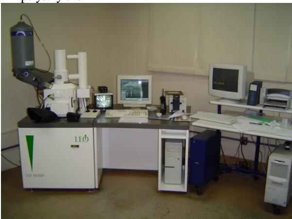
Fig. 5 - Scanning Electron Microscopy – SEM
