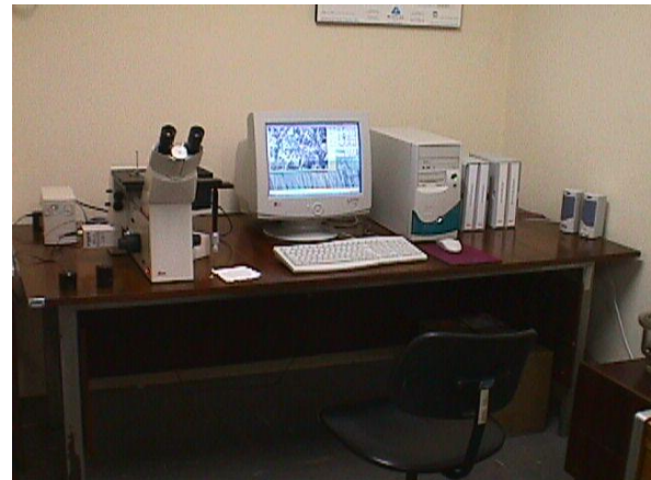
Fig. 6 - Optical microscopy linked to an image analysis system
