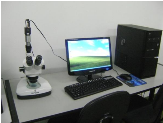
Fig. 4 - Stereoscopic Linked to an Image Analysis System
