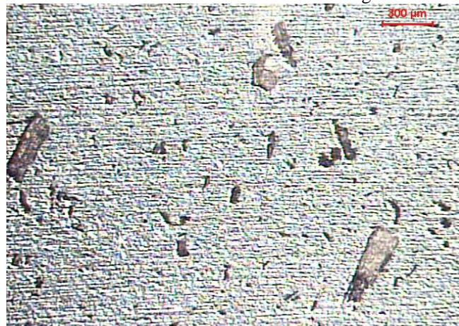
Fig. 8 - Micrography of PP with dispersion with 10% of banana fiber
