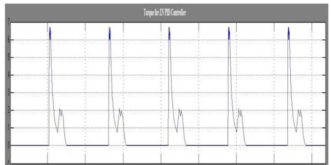
Figure.9. Torque per phase of IM with Z-N PID
