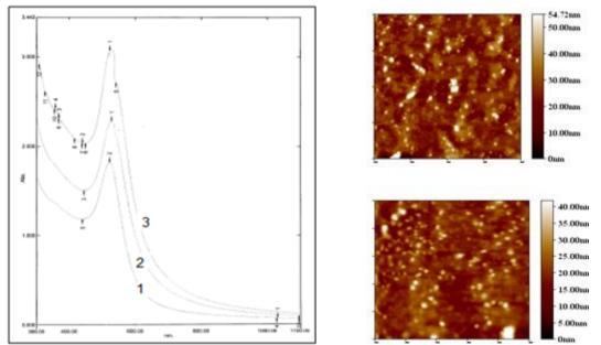
Figure 3: The influence of dialysis and polymer adsorbance on the stability of gold nanoparticles through UV-Vis spectrum and AFM images : curve (1)before dialysis , curve (2) after dialysis and absorbent {2-fold dilution with H2O} and curve (3) without dilution.
