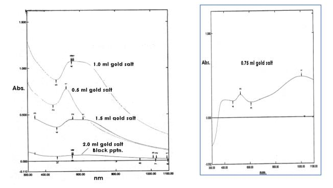
Figure 5: UV-VIS spectrum for the reaction (0.01M) TSC, (0.1M) NaBH<sub>4</sub> with different volumes of (0.01M) HAuCl<sub>4</sub> in order to study the nanoparticles aggregation process.
