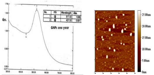
**Figure** 4: UV-VIS spectrum for the stability of GNPs synthesis with method No.3 and AFM image which indicate decreasing in their particle size and stable for one year after dialysis, 0.25µm filtration and polymer absorbent.
