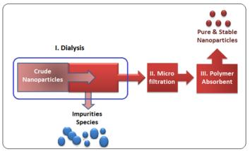
will go through the dialysis membrane (Left). Operation of microfiltration to remove more impurities and sample
