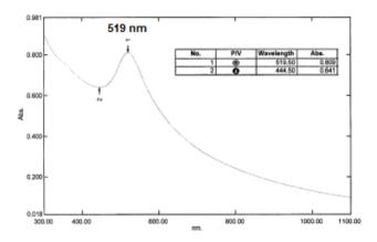
Figure 6: UV-VIS spectrum for the reaction of 0.5ml (0.5 mM) NaBH<sub>4</sub> with 10ml (1.0 mM) HAuCl<sub>4</sub> to produce gold nanoparticles .
