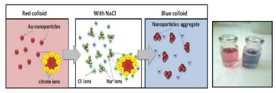
Figure 7: The aggregation of GNPs due to the addition of electrolyte
