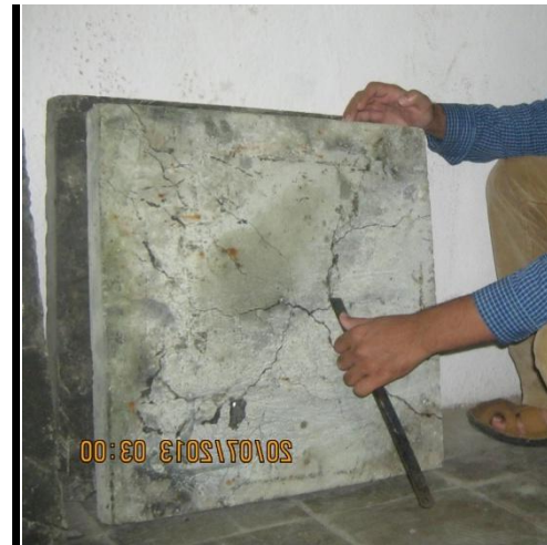
FIG 2. Typical Crack Pattern of HSFRC Slabs after Punching Shear Failure:
