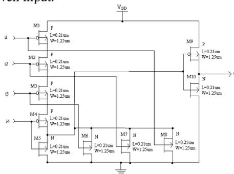
Fig. 3: 4-input OR gate with  $V_{DD}$  as supply voltage
