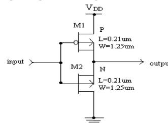
Fig. 1: Inverter with  $V_{DD}$  as supply voltage
