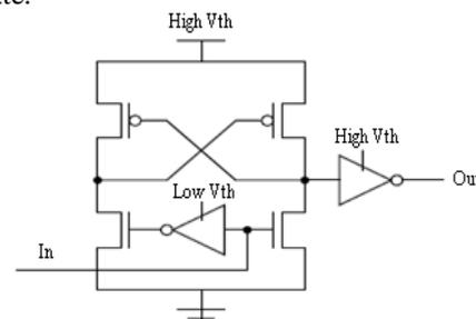
Fig. 8: Differential cascode voltage switched (DCVS) level converter for NOT gate
