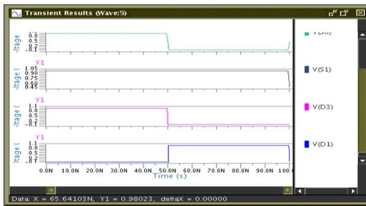
Fig. 11: Simulation waveform of 2x4 Decoder with dual sub-threshold supply voltage
