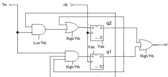
Fig. 12: Moore Machine with dual sub-threshold supply voltage
