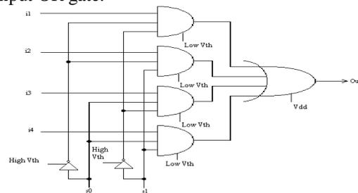
Fig. 6: 4x1 Multiplexer with dual sub-threshold supply voltage
