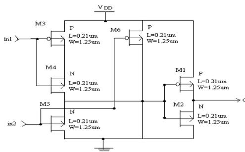
Fig. 4: 2-input AND gate with  $V_{DD}$  as supply voltage.
