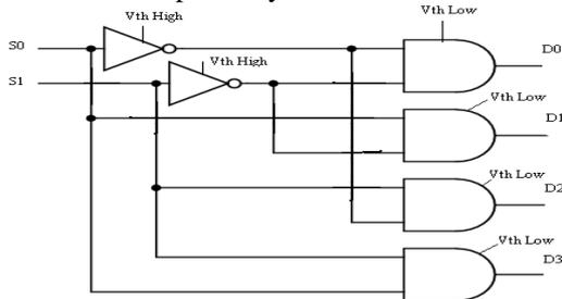
Fig. 10: 2x4 Decoder with dual sub-threshold supply voltage
