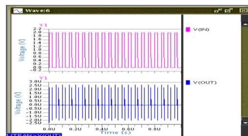
Fig. 9: Simulation waveform of DCVS level converter for NOT gate
