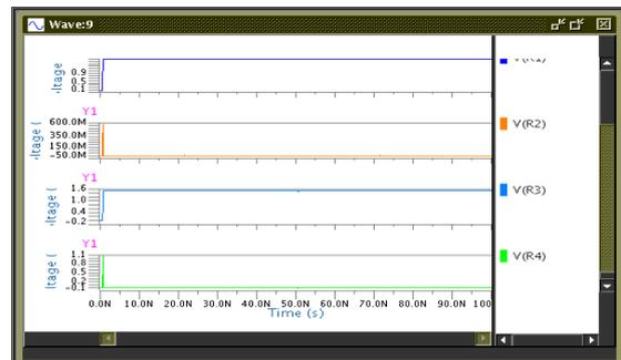
Fig. 15: Simulation waveform of Ring Counter with dual sub-threshold supply voltage
