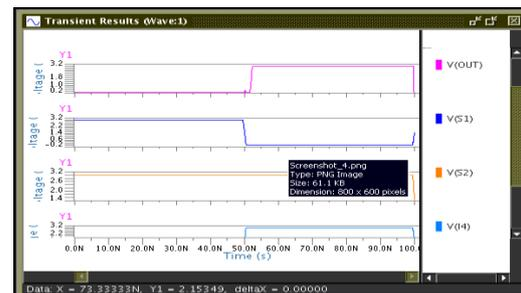
Fig. 7: Simulation waveform of 4x1 Multiplexer with dual sub-threshold supply voltage
