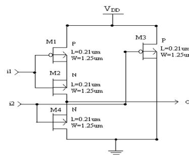
Fig. 2: NAND gate with  $V_{DD}$  as supply voltage
