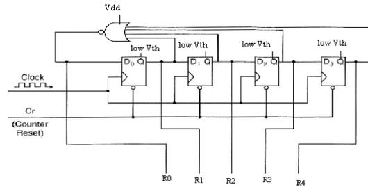
Fig. 14: Ring counter with dual sub-threshold supply voltage
