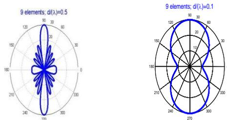
Fig.5: Radiation Pattern of conventional linear array
