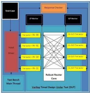
Figure 11 DUT architecture
