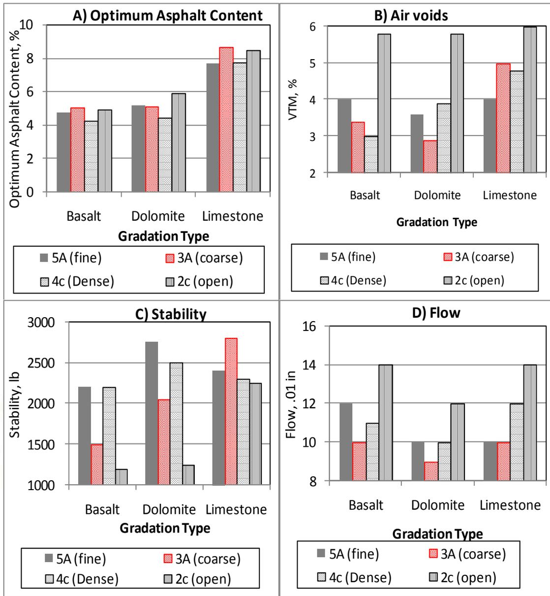
Figure 3 Effect of aggregate type and gradation on mix properties
