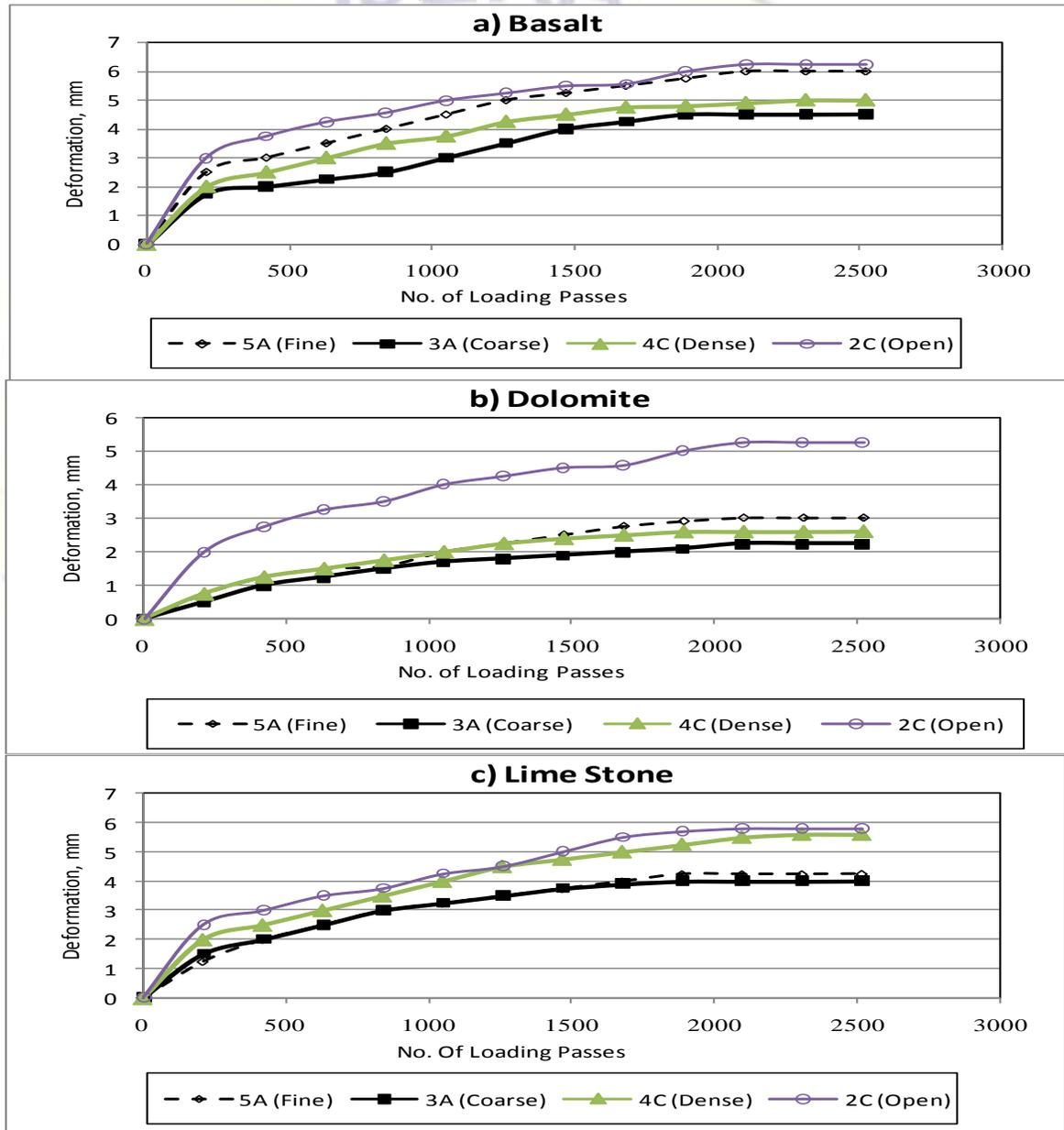
Figure 4 Effect of aggregate gradation on rutting resistance.
