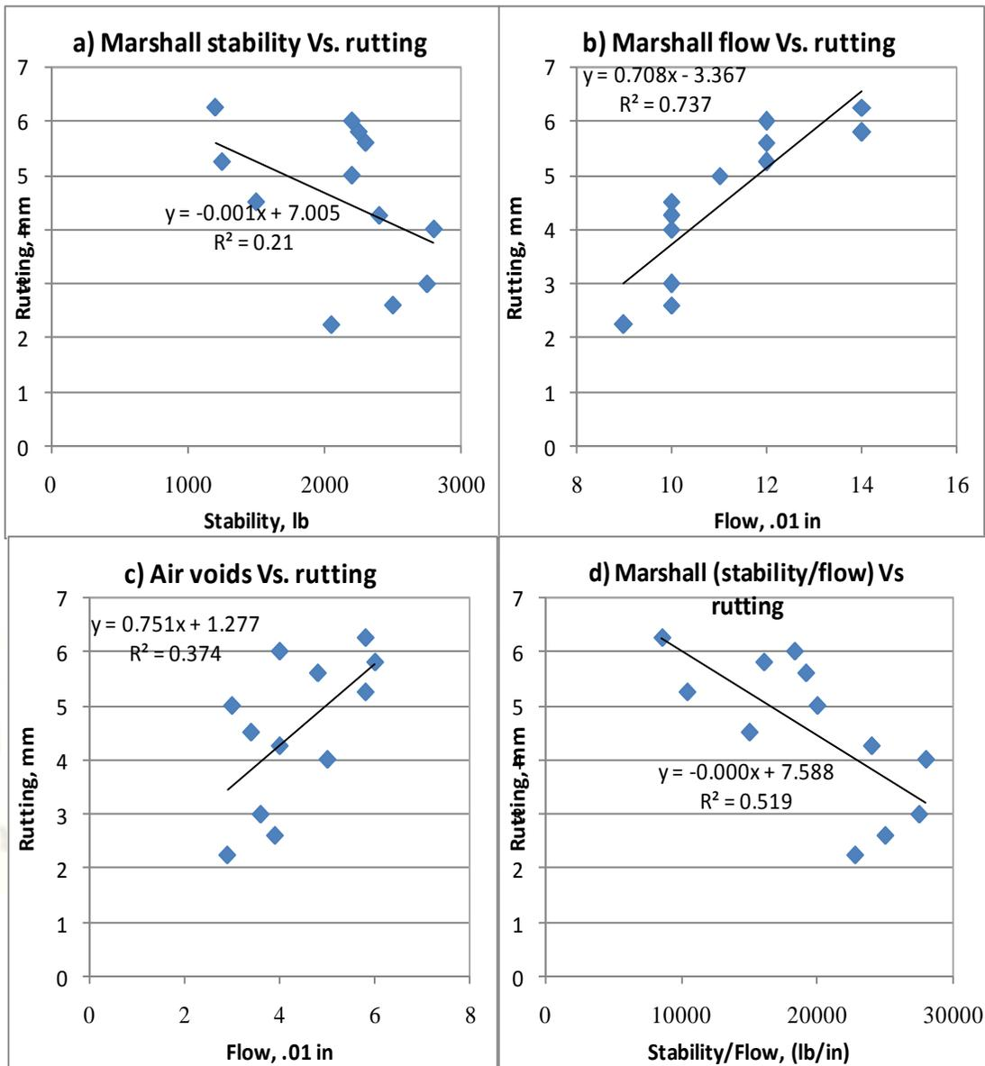
Figure 6 Relation between Marshall mix parameters and rutting
