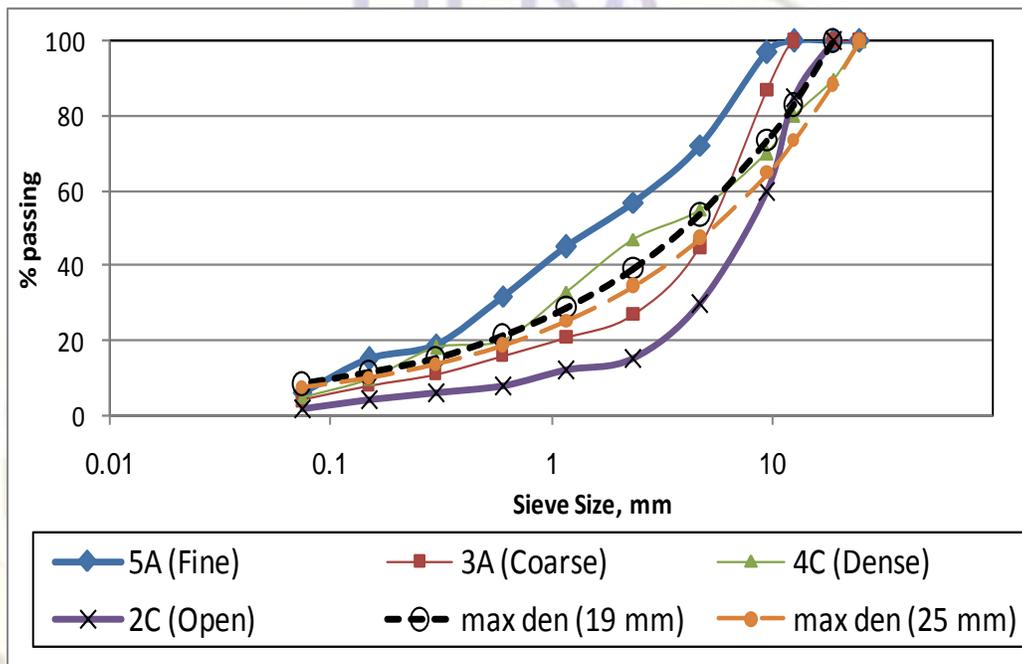
**Figure 1: Aggregate gradation used in the study**
