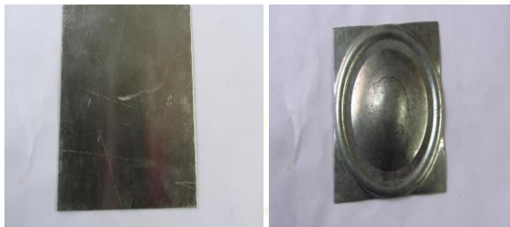
Figure2(a) Figure2(b) a. Soft aluminum specimen before strain analysis b. Soft aluminum specimen after strain analysis
