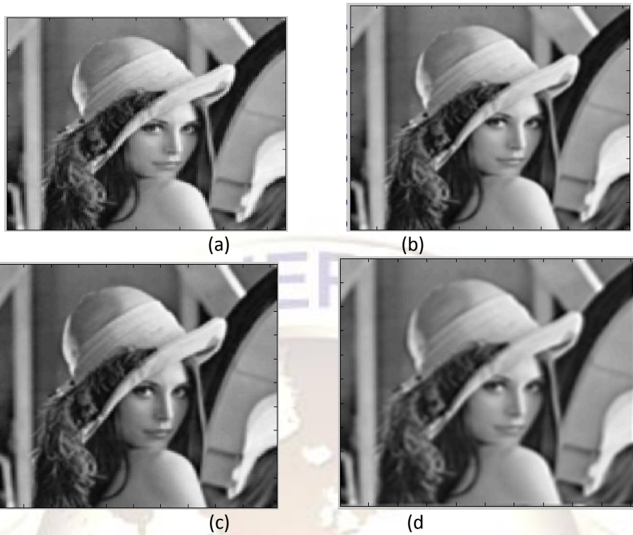
Fig. 6 (a) Lena low resolution image, [b-d] Super resolution methods (b) Interpolation (Bicubic), PSNR=27.62 dB (c) DASR (Db8 + Bicubic), PSNR =24.79 dB, (d) Proposed (Haar + Bicubic), PSNR= 33.08 dB.
