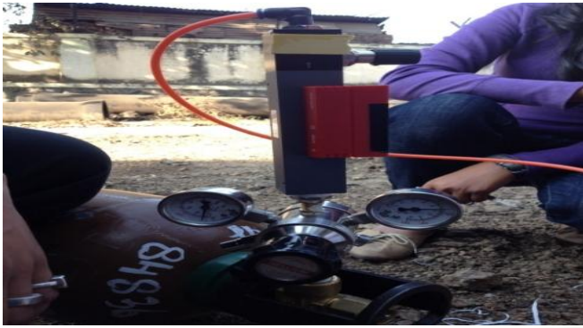
Figure 2.1 Pressure meter with helium gas cylinder
