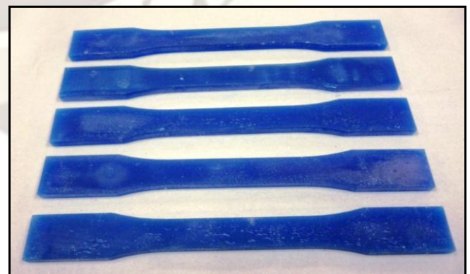
Fig. 2. Dog-bone-shape specimens for tensile test
