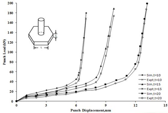
(a) Variation of punch load for 21 mm side of hexagonal head.
