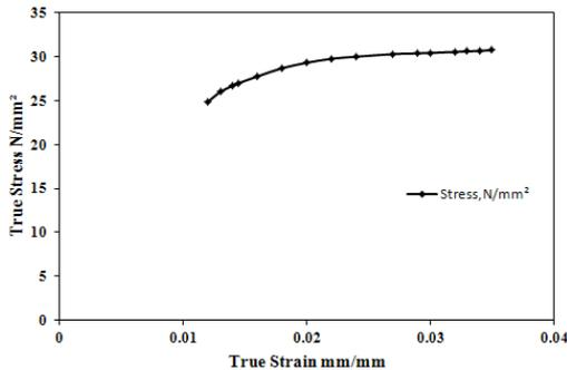
Figure 3. Stress-strain curve for lead.
