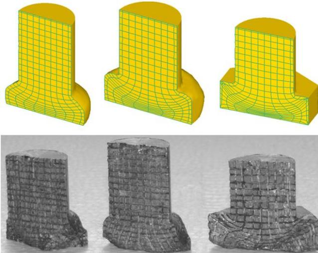
Figure 11. Progressive change of metal flow patterns.
