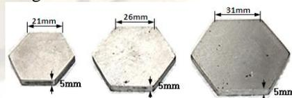
(b) Packing plates used for reduction of die thickness.
